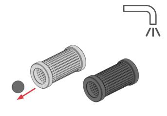
Once the cartridge is clean or replaced, insert the ball inside it;
