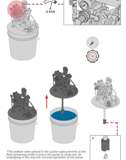
3 Lift up the *diaphragm pump\** together with its connected components;
