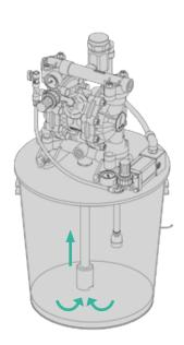
4 At the same time with the first, the movement of the second diaphragm *pushes* the fluid inside the pump to flow by the outlet. These two actions are repeated cyclically and alternately by the two diaphragms, producing in this way a continuous flow;
