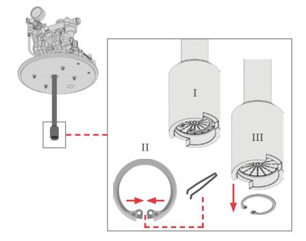
3 Then pull out the *filter* from the bottom valve;
