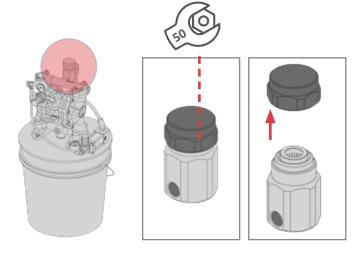
2 Look inside the cap to check the wear of the gasket and if it is necessary, replace it;
