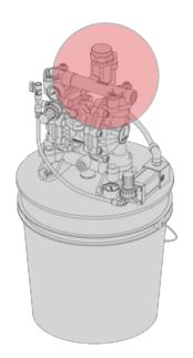
Then the filtered fluid flows through a fitting into the *fluid pressure regulator* [pos.8]. Depending on the adjustment position of the the fluid pressure regulator, this component operates on the fluid inlet, regulating the outlet pressure according to the needs.
