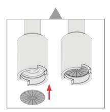
6 With the help of a pair of tweezers insert the *snap ring* in the internal seat;
