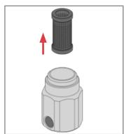
Pull out the *ball* and rinse with water. Put the *filter cartridge* under running water to remove any lumps and sedimentation. Then blow with compressed air to clear the meshes from any impurities still present. If these operations become difficult or ineffective, is necessary to replace the component;
