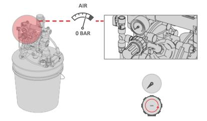
3 Lift up the diaphragm pump\* together with its connected components;
