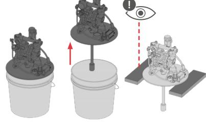
Fill the bucket with the desired fluid\* (max 28 litre), then reposition the diaphragm pump and check the correct positioning of the lid along the edge of the bucket;
