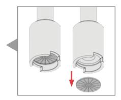
Put the *filter* under running water to remove any lumps and sedimentation. Then blow with compressed air to clear the meshes from any impurities still present. If these operations become difficult or ineffective, is necessary to replace the component;
