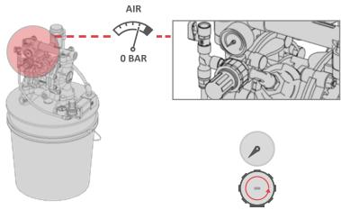
14 Once the water no longer comes out from the nozzles of the *dispensing valves*, the fluid inside the system is no longer under pressure. Then is possible turn off the valves;
