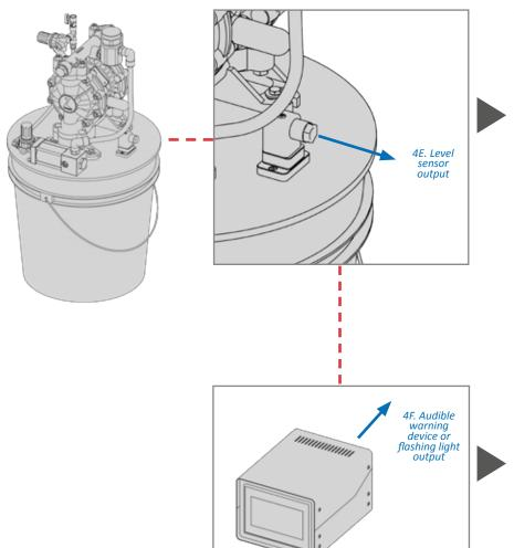
The *level sensor* must be connected by a Zator's microprocessor control or alternately by an instrument tested and approved by Zator.
