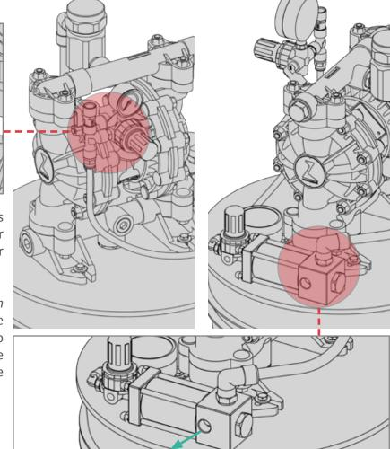
A *flexible plastic pipe\** for use **up to 6 bar** must be connected to a proper *G3/8" fitting\** to be screwed on the filter outlet.
