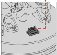
2. Screw the connector screws;
