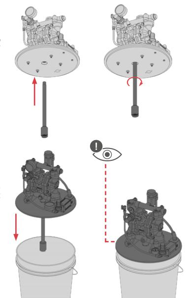
2. Place the *diaphragm pump* and check the correct positioning of the *lid* along the edge of the bucket.
