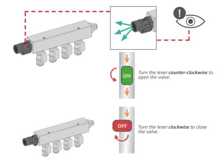
10 Turn on the *dispensing valves* allowing the fluid to come out from the nozzles;
