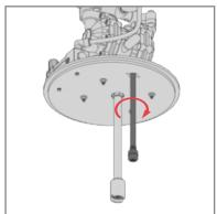
4. Insert the *female connector* of the level sensor;
