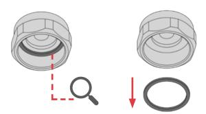
3 Pull out the *cartridge* of the filter/ pulsation dampener **being careful** not to drop the ball placed inside it because it is free to move;
