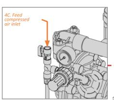
The double diaphragm pump for its functioning needs compressed air coming from an external plant for the production and distribution.
