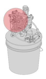
**2** From the *pressure regulator* the air flows inside the pump, activating the two internal diaphragms. These two diaphragms move together and produce two different actions on the fluid;
