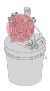
The movement of one of the two diaphragm cause the *vacuum effect* inside the *suction pipe* [pos.6]. This action allows to the fluid to be extracted from the bucket and goes up through the pipe inside the pump. The mesh filter inside the *bottom valve* [pos.7] prevents the aspiration of any possible lumps and contaminants contained in the fluid;
